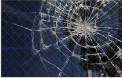
BREAKAGE PATTERN OF LAMINATED GLASS
