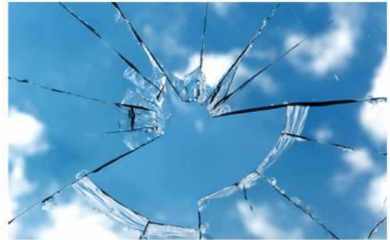
Breakage pattern of HS Glass
