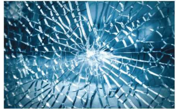
Breakage Pattern of Toughened
